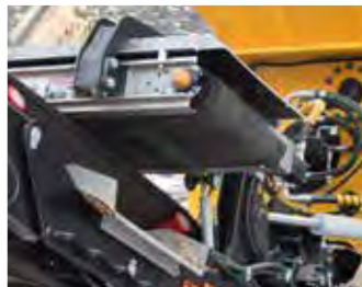
Overband magnet separates metals. (option)
