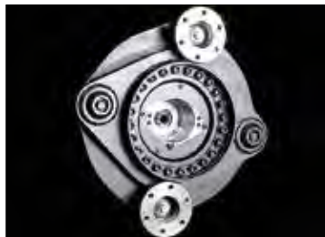
Rotor carrier assembly, swing frame (pat.) protects the gears.
