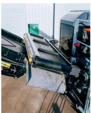
High strength overband magnet with hydraulic height adjustment (Optional)
