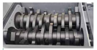
Expertly designed in-house shredding chamber 2 x 1.5m long shafts made from heavy duty steel with welded teeth
