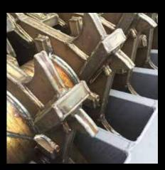
Shaft cutting elements are a fully welded structure with hard-faced edges giving ultimate strength in difficult applications
