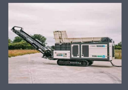
and noise the TDS 820e replaces the Scania DC13 diesel engine with a powerful 280kW WEG electric motor. This change also results in reduced maintenance time and costs. The TDS 820e is fitted with a small 55kW CAT C2.2 engine for tracking and machine set-up, resulting in minimal down time.
