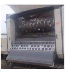
Medium speed shredder with aggressive cutting teeth
