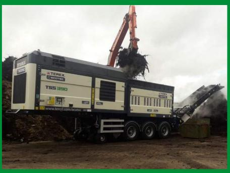
The TSS 390's 3m long shredding shaft was expertly designed in-house and is made from heavy-duty steel, with easily replaceable, bolt-on shredding teeth. Being hydrostatically driven, it offers the benefit of full speed, full torque reverse as well as protection against contaminants. Customisable shredding programs enable the operator to configure the machine to their specific requirements and offers improved shaft cleaning in difficult applications, reducing wrappage and optimising throughput.
