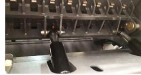
Hydraulically adjusted counter comb allowing product size to be altered to requirements
